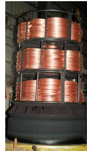
Eddy Current tested LWC / Jumbo Coils are wound and weight 100 kg approximately.
